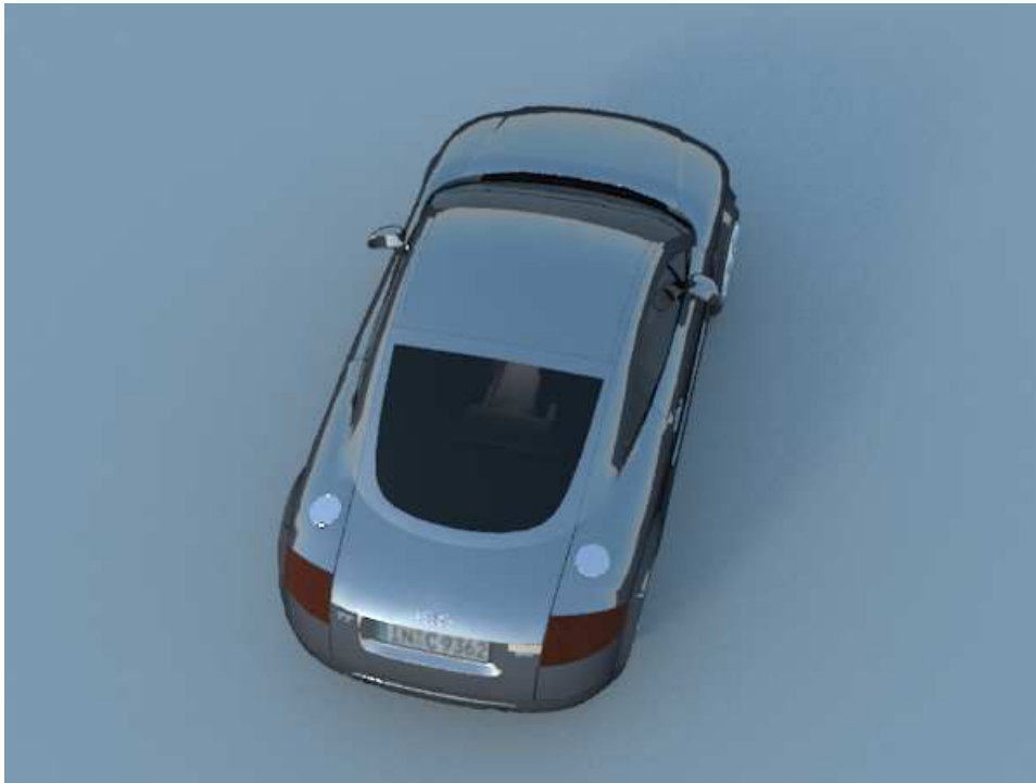
Figure 2: TT car model illuminated by the morning skylight environment map, rendered with four image samples per pixel and eight light source samples per image sample. The top image shows the result from using a uniform sampling distribution, while the bottom image shows the improvement from the method implemented here. Note that a total of just 32 light samples per pixel gives an excellent result with this approach.
